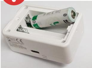
The sensor works with 1 or 2 batteries of type ER14500, these have a nominal voltage of 3.6 V and a capacity of 2600mAh. Operation is parallel, which means that the batteries are inserted in identical positions. Ensure that **the negative pole is on the metal spring inside the battery compartment, the positive pole with the round, flattened tip must be on the flat battery contact.**
