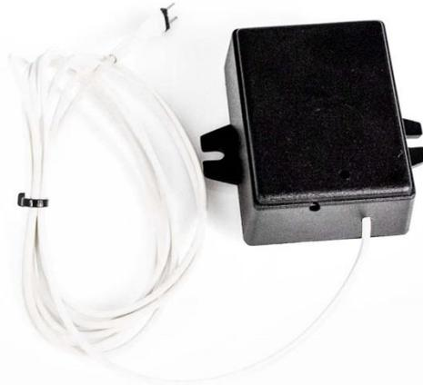
**Sensors ordered in sets are sent already connected/programmed to the Direct-Smarter Android Alarm Center/Connector. Please, first clean the surfaces (with alcohol or glass cleaner) to which the sensors are attached. To attach the TC Circuit housing, please use the adhesive pad.**
