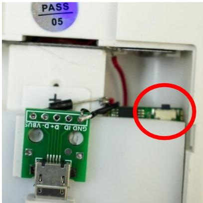
After the camera has been successfully connected, slide the slide switch (remove the rear cover → bottom right) from the right position to the left position with the black dot so that the camera can only be switched on via the AIS Center. This ensures that only you and no one else can access the camera.
