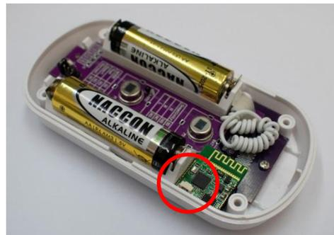
The motion detector is used to monitor rooms. The sensor has an 80-degree lens and a detection range of approx. 8 meters / 26 feet.
